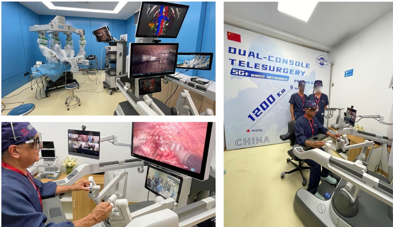
Fig. 1 Physician performing telesurgery on animal mode 1200 km away in china. Surgeon console contains miniature screen of remote site control room and operating room
